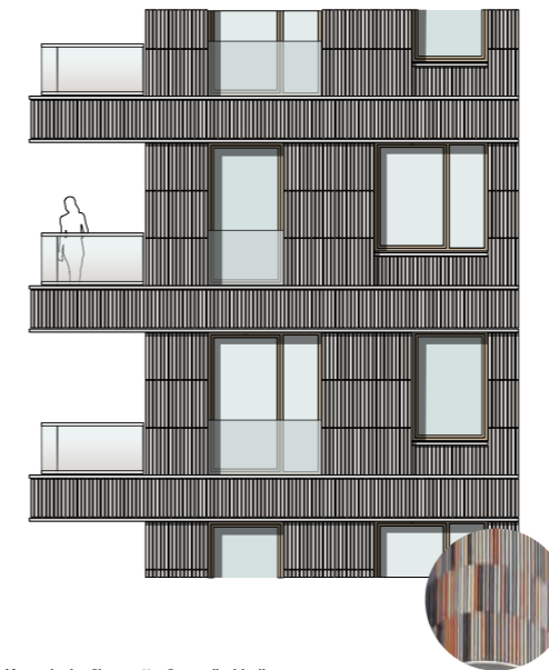
Keramische “baquettes” gevelbekleding.
